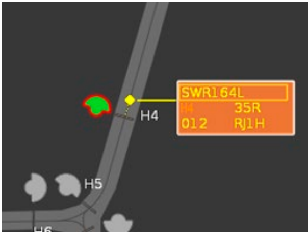
Figure 6. Unauthorized Stop Bar Crossing
