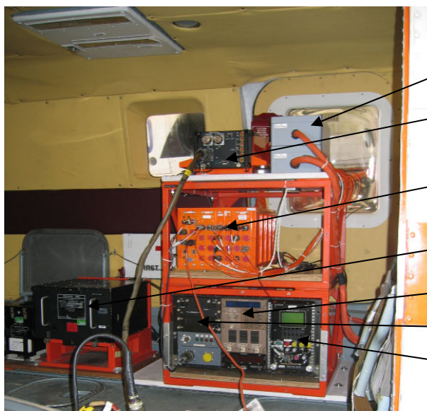
Figure 4: The ring laser gyro and measurement system in the KA32T
