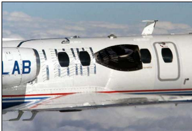
Figure 12-2: Photo of the tufts showing the air flow behind the fairing on the Citation.
