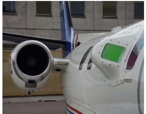
Figure 12-3 Fairing on the NLR Cessna Citation II housing the mirror deflecting the I-Wake laser beam to the measurement volume in front of the aircraft and receiving scattered light. On the two pictures on the left side tufts are attached to the fairing and aircraft to study the influence on aerodynamics. In the picture above the final coating has been applied
