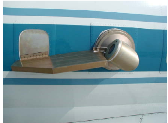
Figure 6: Lidar turning mirror faring in stowed position on the NASA DC-8 aircraft [30].
