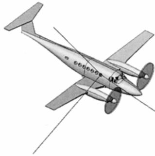
Figure 9: Beechcraft King-air showing MOADS laser beams projected from a side fuselage window [32].
