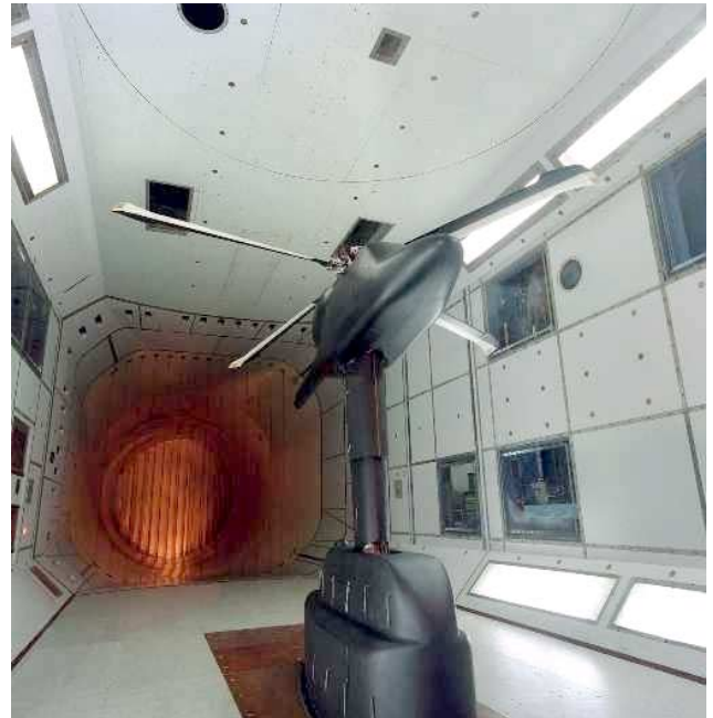
Rotor test rig and experimental rotor in QinetiQ 5 Metre Wind Tunnel, from HC(AG) on 'Validation of rotor blade / hub load synthesis techniques'
