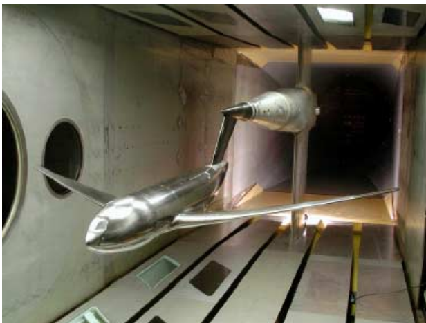
Aérospatiale AS-28 model in DNW-HST High Speed Wind Tunnel test-section, from AD(AG) on 'Transonic wing/body code validation experiment'
