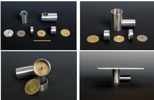
Figure 2: Photos of a 3DOF air-injected acoustic liner sample
