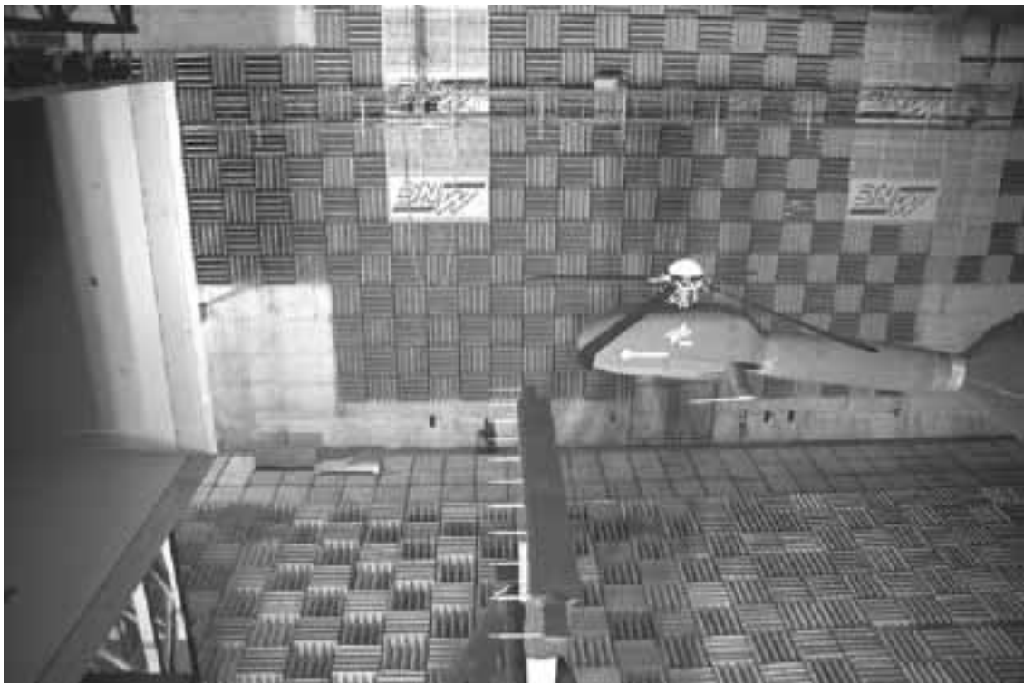
Fig. 27 Helicopter noise test set-up in DNW
