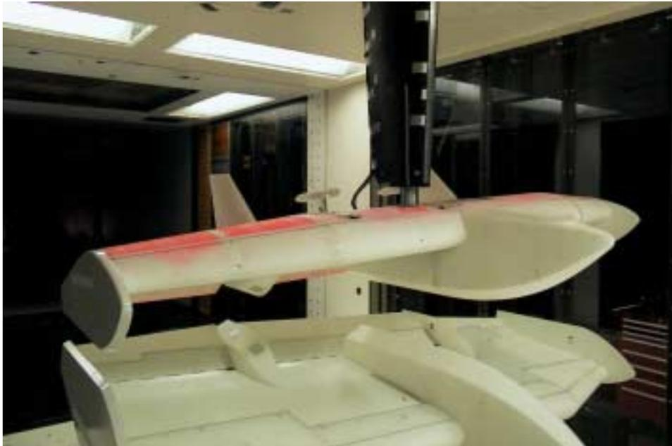
*Fig. 5 Seabus wind tunnel models with 30° flap deflection*
