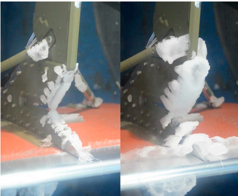
Figure 10: Ice accretion on unheated scissor at -10^{\circ}\text{C} after 5-min (left) and 30-min (right) CMI exposure at high-speed cruise conditions.
