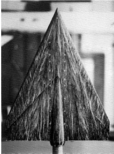
Fig.27 Oil flow visualization indicating attached conical flow close to the leading edge followed by shock induced separation and vortex formation; supersonic leading edge, 65 deg delta wing with rounded leading edge, Mach= 2.18, \alpha= 8 degrees (Elsenaar, 1988)
