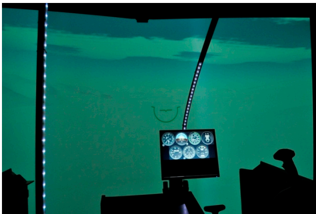
Figure 7 View from the cockpit in the CFIT scenario with the HUD Orange Peel and LED concept
