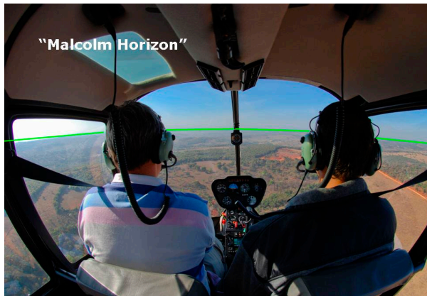
Figure 2 Extended horizon line or Malcolm Horizon (MH) concept
