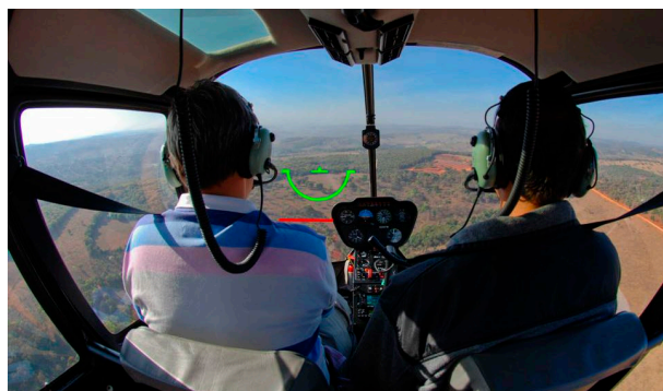
Figure 3 Head-Up Display (HUD) of attitude recovery using the “Orange Peel”
