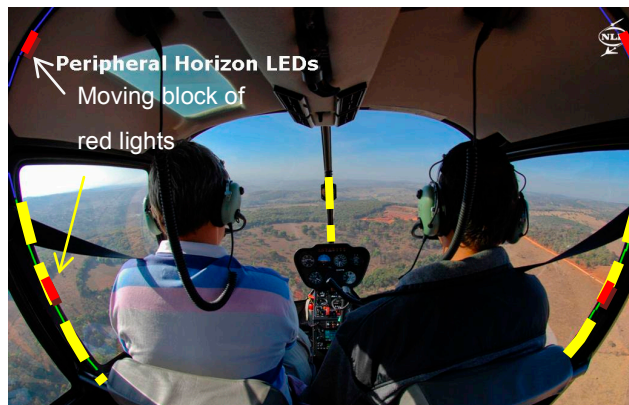
Figure 5 LED lights mounted in the peripheral view of the pilot
