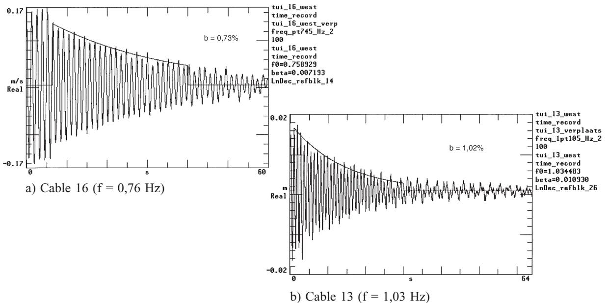
Fig. 7 Decay of cable with prototype dampers and the curve-fit procedure (LnDec)
