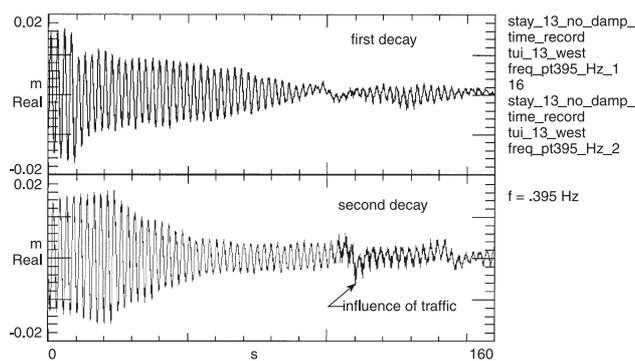
Fig. 6 Conflicting decay's of cable 13 without damping devices
