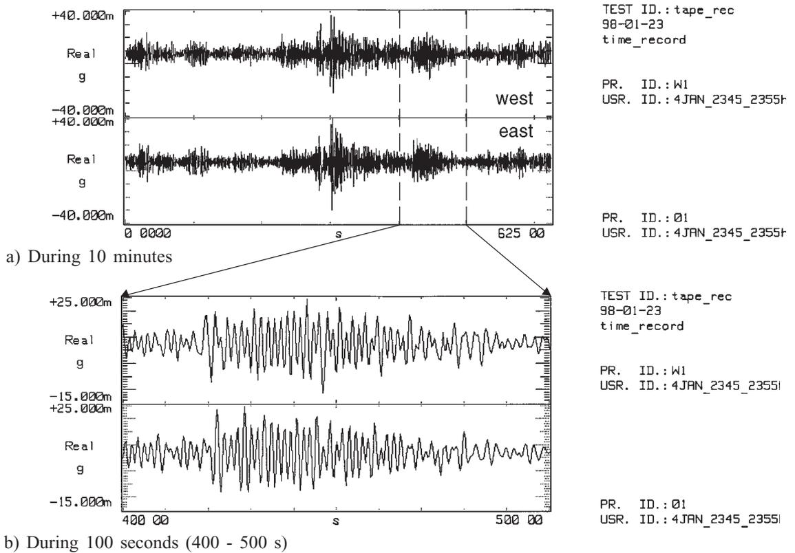
Fig. 11 Example of time signals of accelerometers (east and west)
