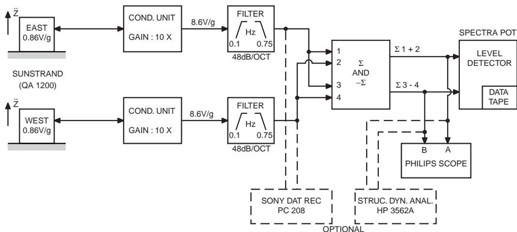
Fig. 9 Diagram of monitoring equipment
