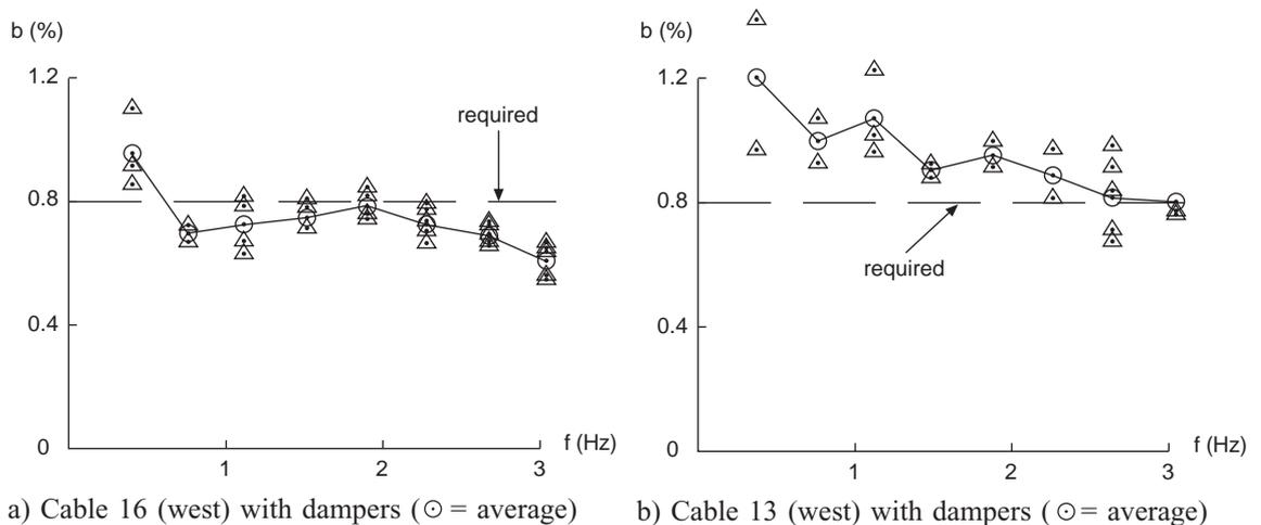
Fig. 8 Damping obtained with prototype dampers
