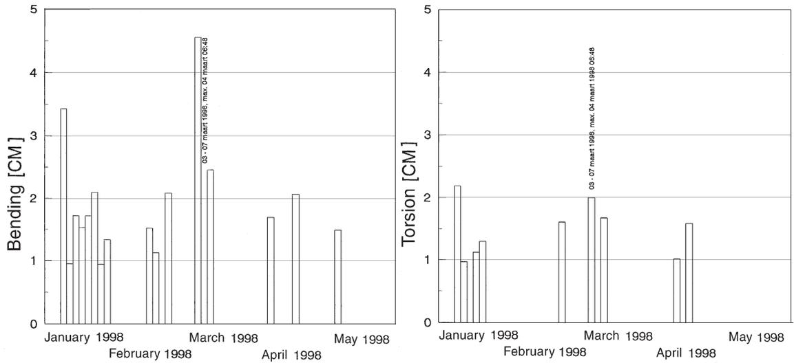
Fig. 10 Results of monitoring (amplitudes peak to peak) at the position of railing
