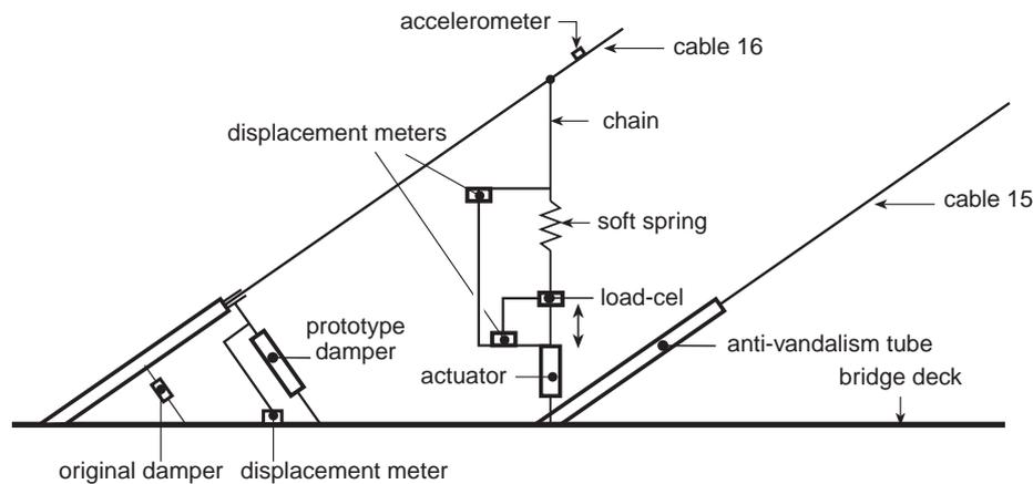
Fig. 5 Hydraulic Actuator System
