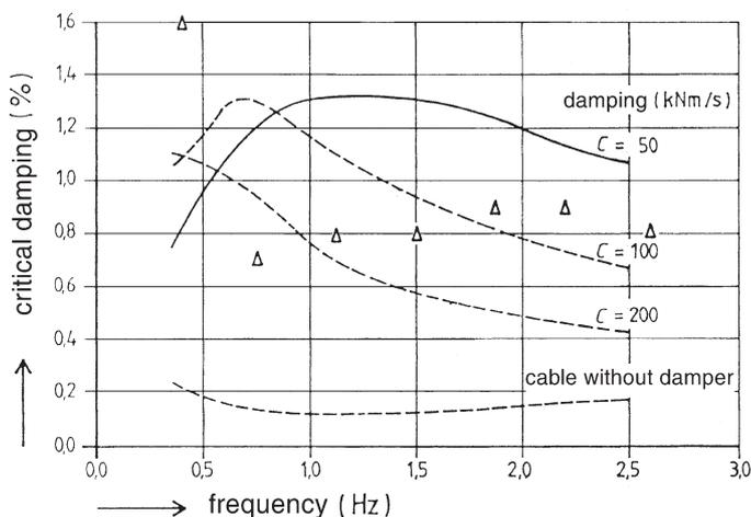
Fig. 3 Calculated and measured ( $\Delta$ ) damping values
