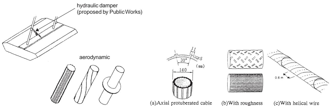
Fig. 2 Aerodynamic counter-measures to prevent cable vibrations
