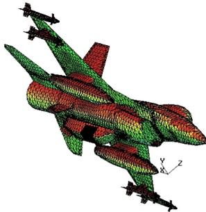
Figure 3 Geometrical approximation of the exterior surface of the aircraft
