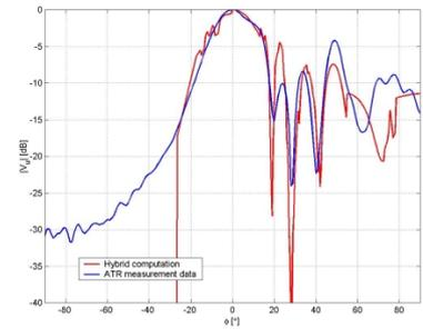
Figure 5 Computational results compared with antenna measurements (horizontal polarisation)
