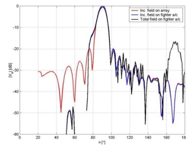
Figure 8 Computational result for SAR antenna on pod
