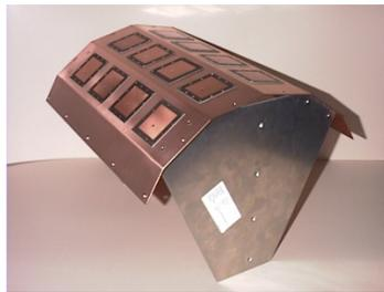
Figure 2 Conformal antenna array of 16 microstrip patch elements
