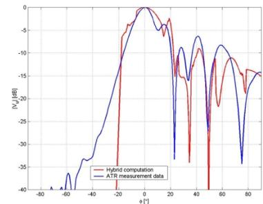
Figure 6 Computational results compared with antenna measurements (vertical polarisation)
