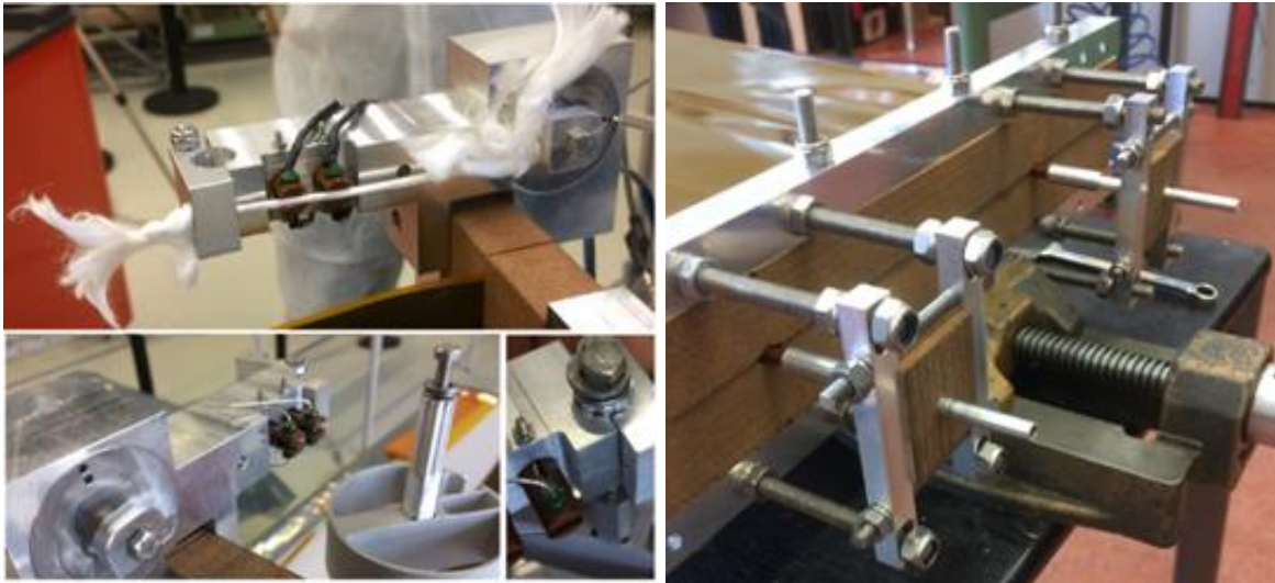
Figure 12. Hold-Down and Release Mechanism (HDRM, left), Foil Radiator Fixation (FRF, right)
