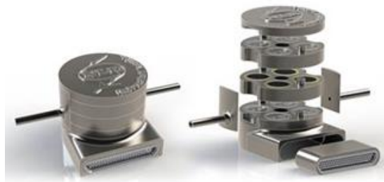
Figure 8. Multi-parallel micro-pump under development at NLR
