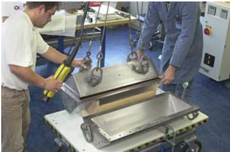
Fig. 6 Positioning the inner mould (including pre-form and core mandrel) into the outer mould.
