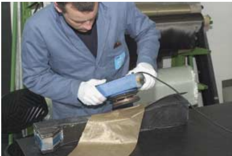
Fig. 4 Making the pre-form on the core mandrel
