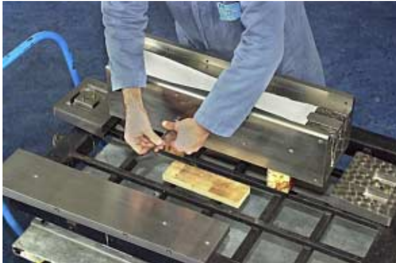
Fig. 5 Positioning the pre-form and core mandrel into the inner mould
