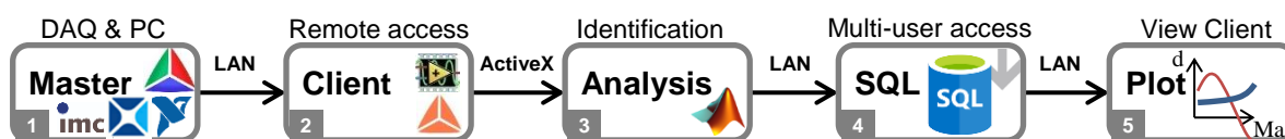
Figure 25: Dataflow of online monitoring process.
