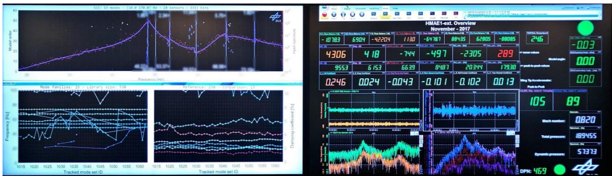
Figure 24: Displays in control room: modal parameters (left) and balance signals (right).
