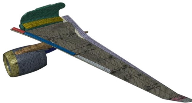
Figure 6: Abaqus FE-model of the wing.
