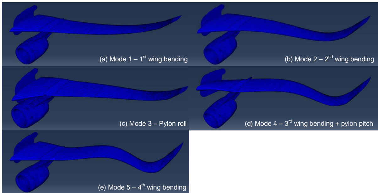
Figure 18: First five mode shapes (free-free conditions) as determined with the detailed Abaqus model.
