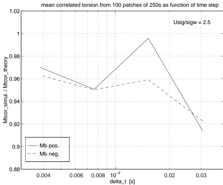
Fig. A.17 A310 mean correlated torsion from 100 patches of 250 s as function of time step, for two turbulence intensity levels
