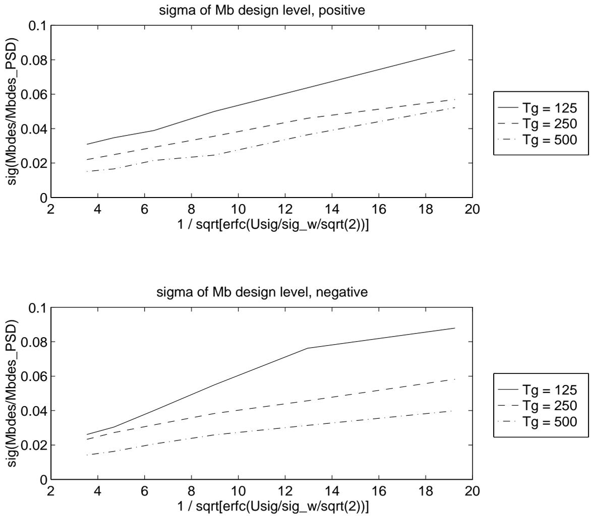
Fig. A.3 Linear A310 bending moment design level standard deviation as function of turbulence intensity  $\sigma_w$
