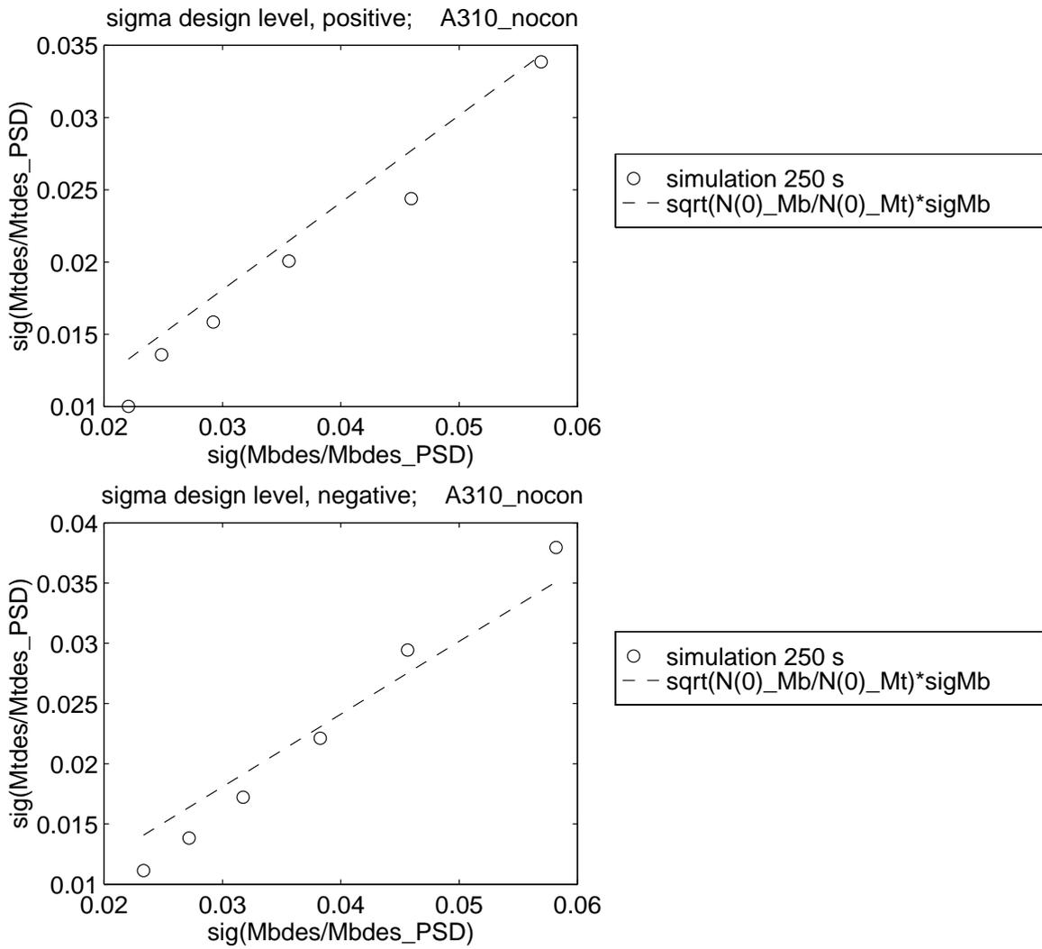
Fig. A.6 A310 torsion design level standard deviation as function of bending design level standard deviation
