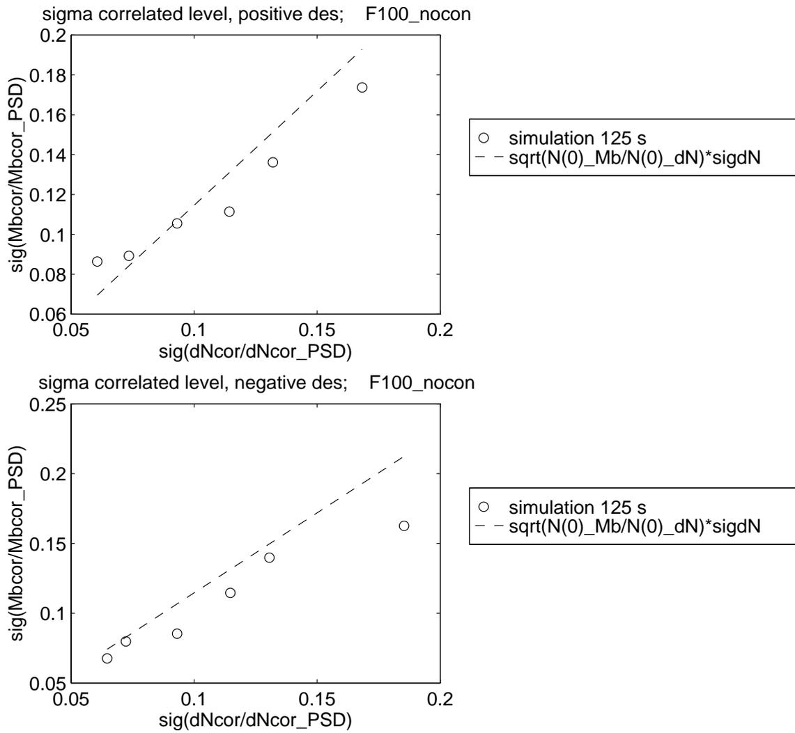
Fig. A.14 F100 bending correlated level standard deviation as function of load factor correlated level standard deviation
