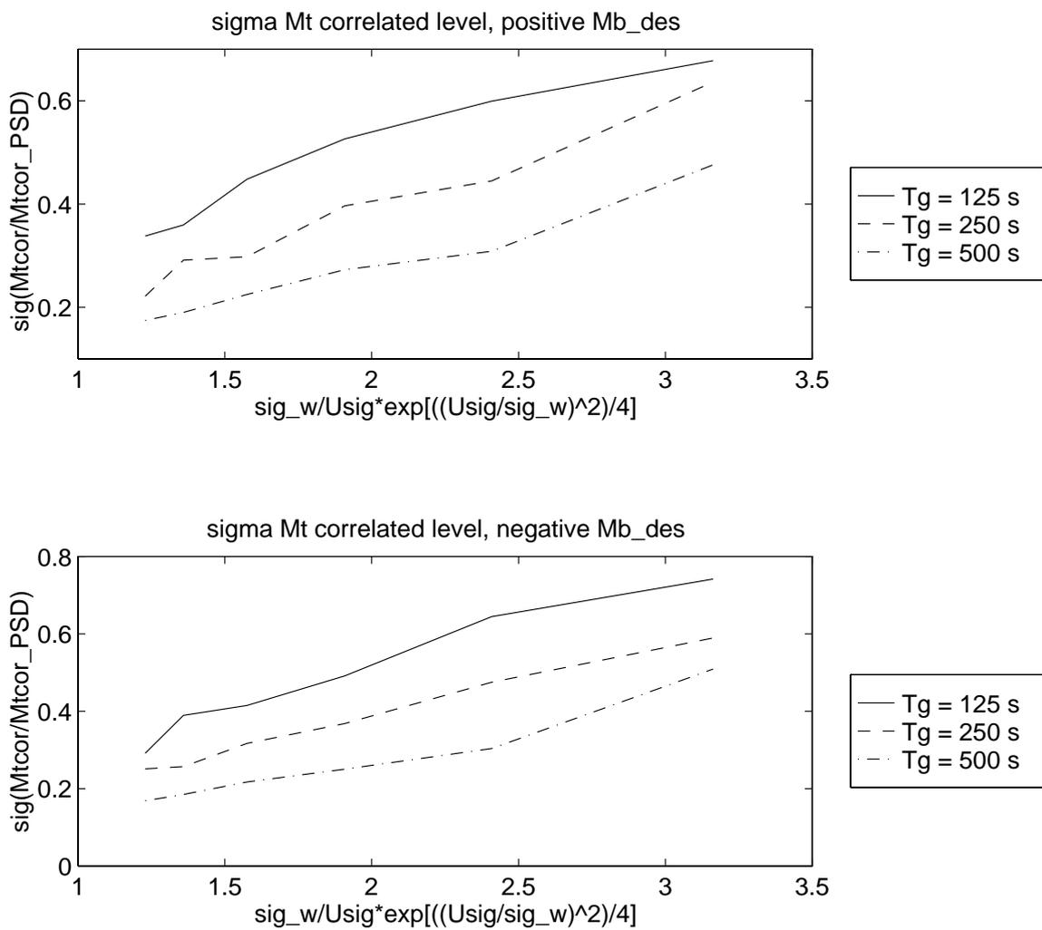
Fig. A.12 Linear A310 torsion moment correlated level standard deviation as function of turbulence intensity  $\sigma_w$
