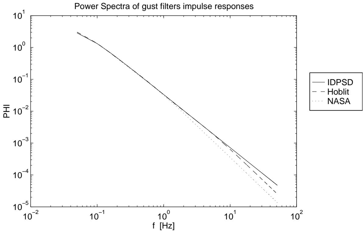
Fig. 7 Power Spectra of three gust filters impulse responses
