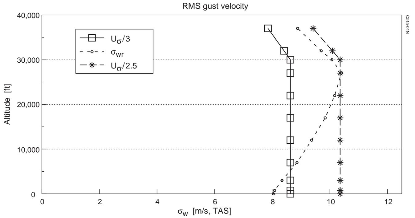
Fig. 2 Three functions of rms gust velocity versus altitude
