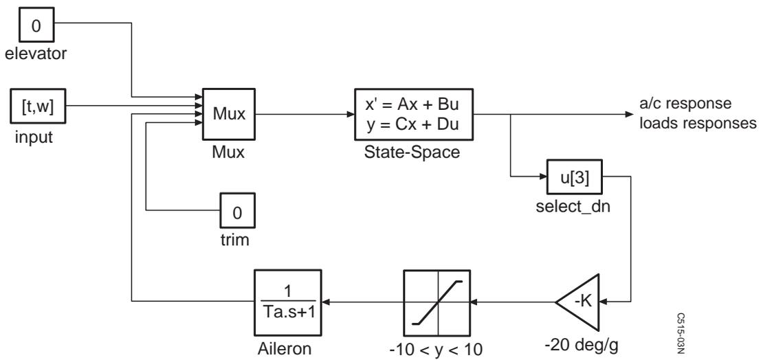
Fig. B.2 Fokker 100 aircraft model with load alleviation using ailerons (Ref. 6)
