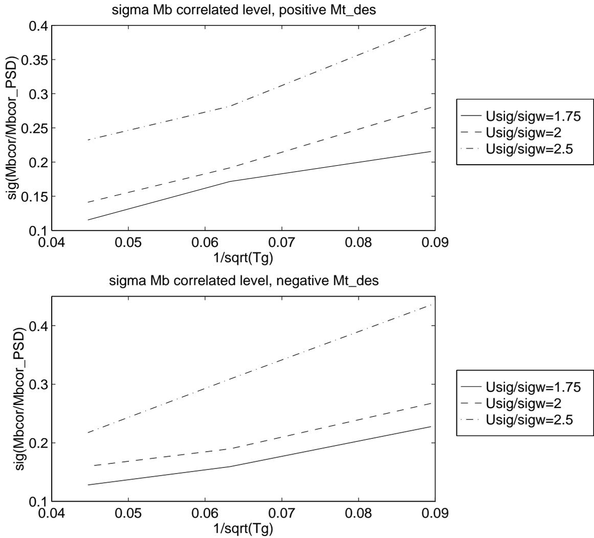
Fig. A.9 Linear A310 bending moment correlated level standard deviation as function of turbulence patch length
