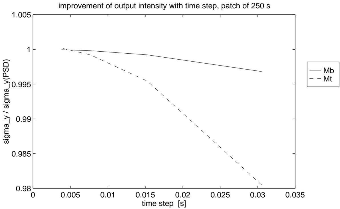
Fig. 6 Improvement of A310 output intensity with time step with respect to theoretical PSD value
