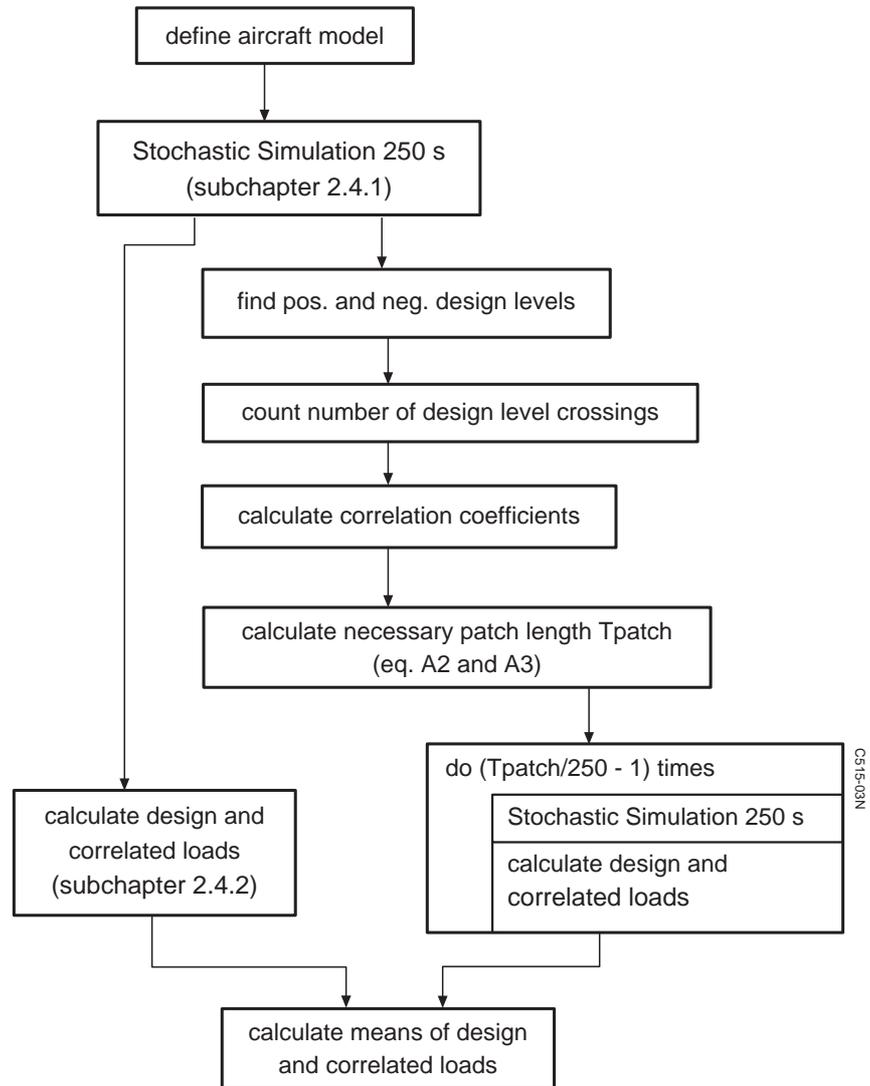
Fig. A.18 The proposed Stochastic Simulation procedure
