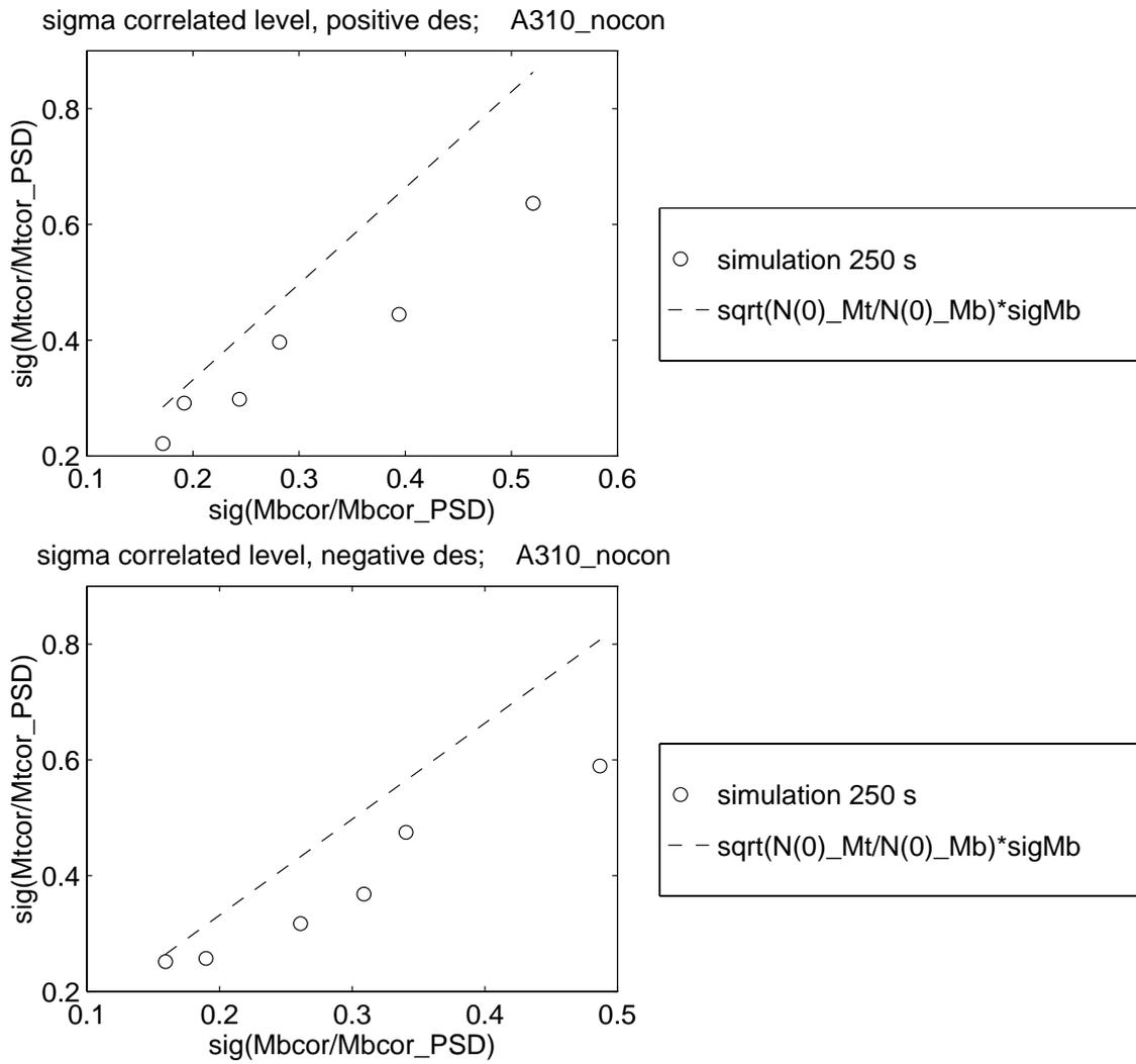
Fig. A.13 A310 torsion correlated level standard deviation as function of bending correlated level standard deviation
