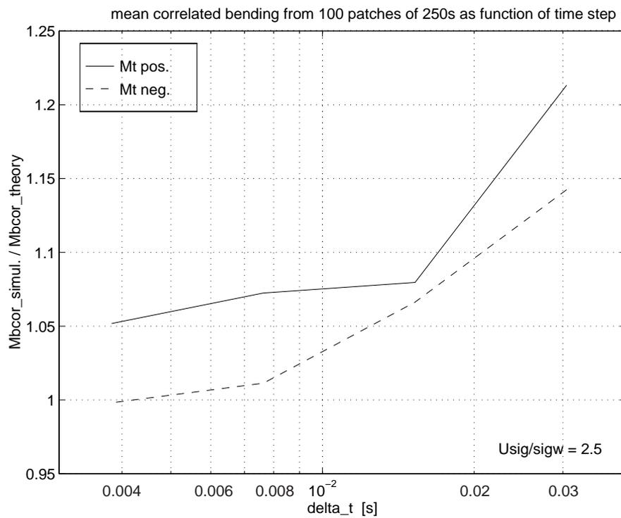
Fig. A.16 A310 mean correlated bending from 100 patches of 250 s as function of time step, for two turbulence intensity levels
