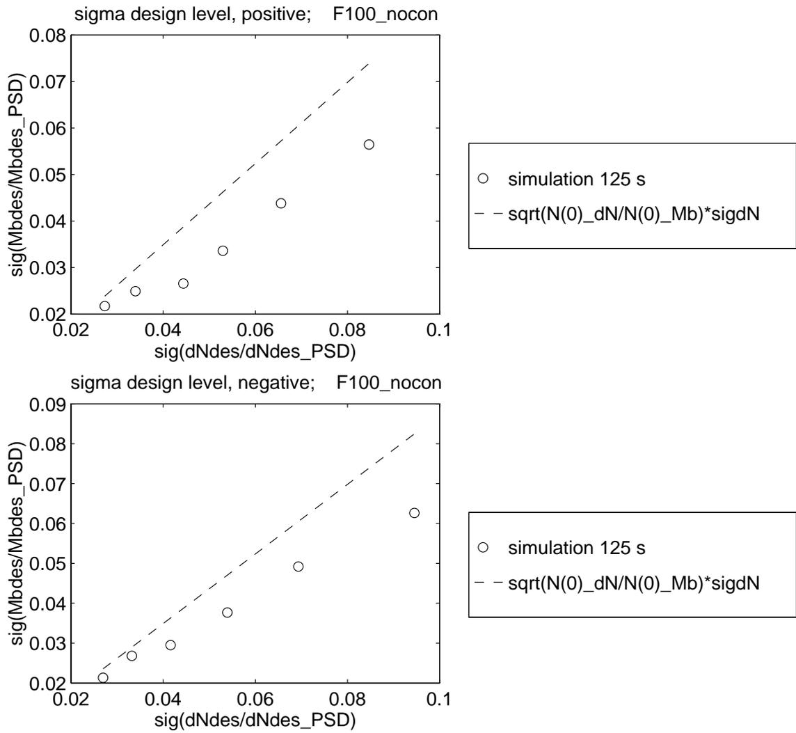
Fig. A.7 F100 bending design level standard deviation as function of load factor design level standard deviation
