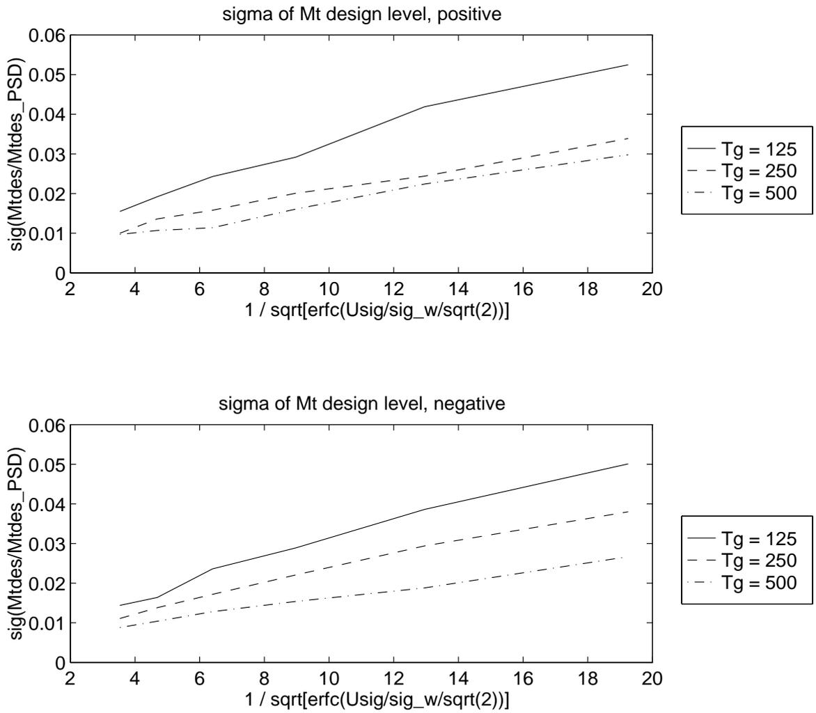
Fig. A.4 Linear A310 torsion moment design level standard deviation as function of turbulence intensity  $\sigma_w$
