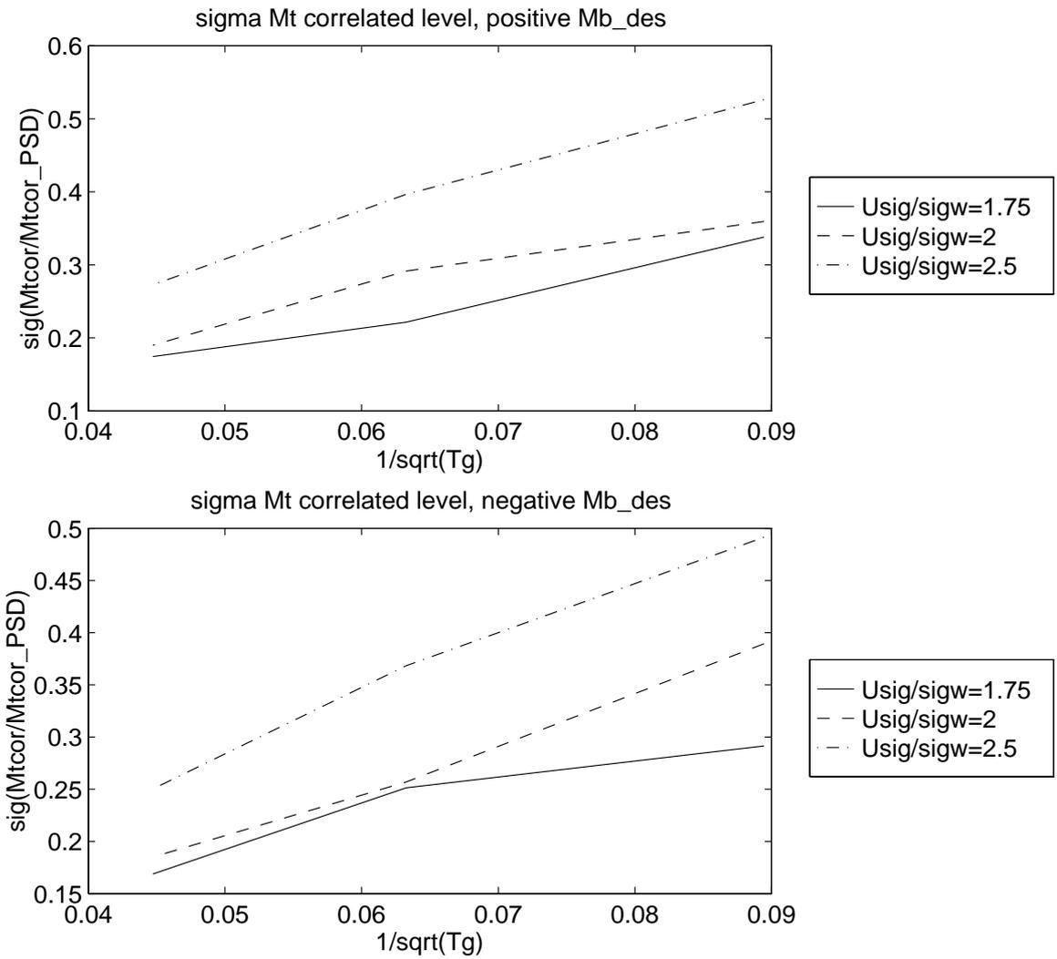
Fig. A.10 Linear A310 torsion moment correlated level standard deviation as function of turbulence patch length
