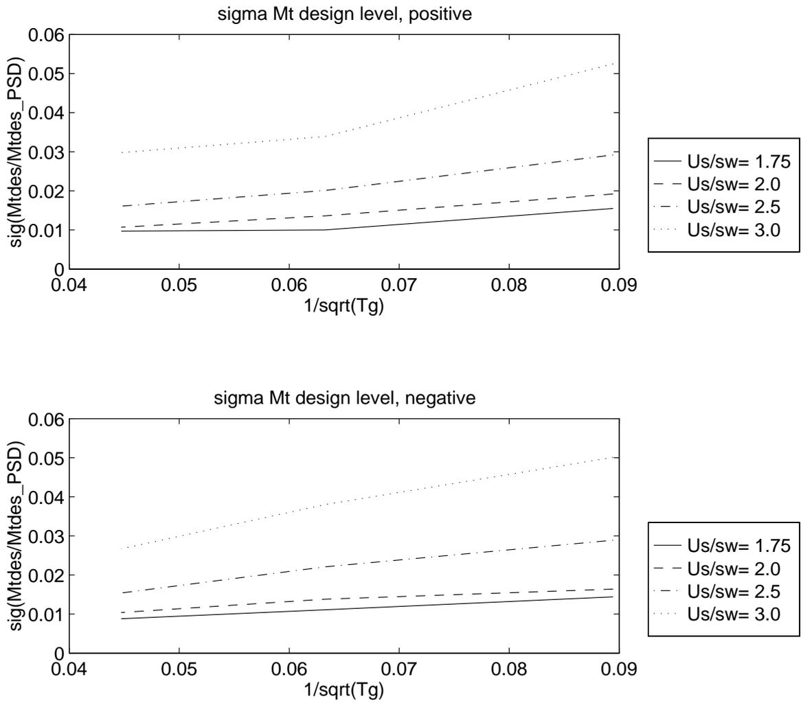
Fig. A.2 Linear A310 torsion moment design level standard deviation as function of turbulence patch length
