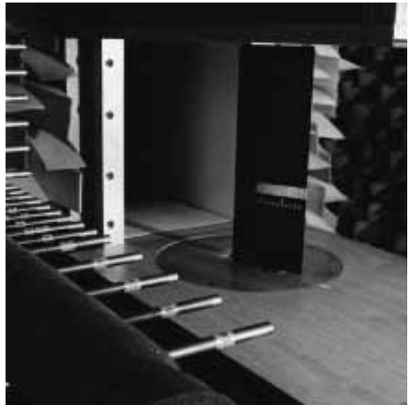
*Fig.1 Acoustic antenna set-up for airfoil self-noise measurements in Small Anechoic Wind Tunnel*
