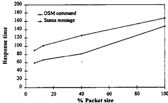
Figure 3 Measured response times with 149 Mbps ATM with nominal workload
