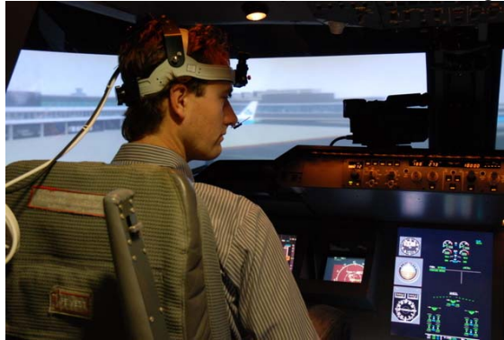
Fig. 2. Combining data streams. Pilot in simulator while several tools (e.g. eye tracker IR camera) are registering data.
