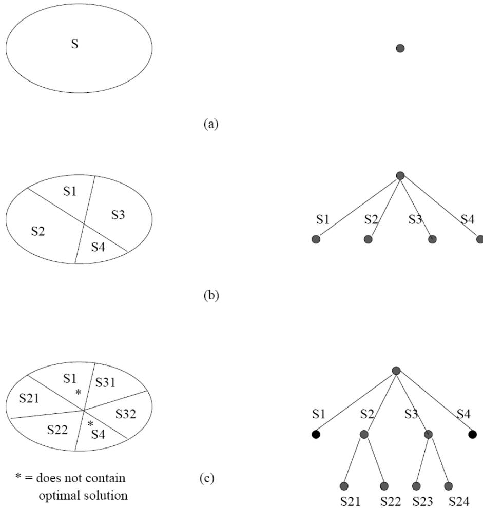
**Fig. 17** Illustration of the tree structure created from a design set  $S$  with the branch-and-bound method. The set  $S$  of possible solutions is partitioned. Subsets  $S_1$  and  $S_4$  are not further subdivided in a tree structure because a bound function indicates that they do not contain the optimal solution (picture from Ref. 10).
