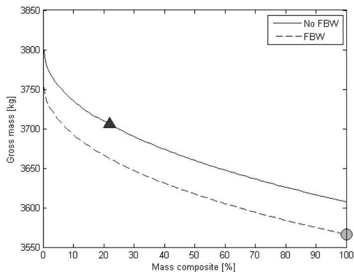
**Fig. 20 Minimum helicopter mass (circle) found for 100% composite mass in the fuselage and a fly-by-wire flight control system**
