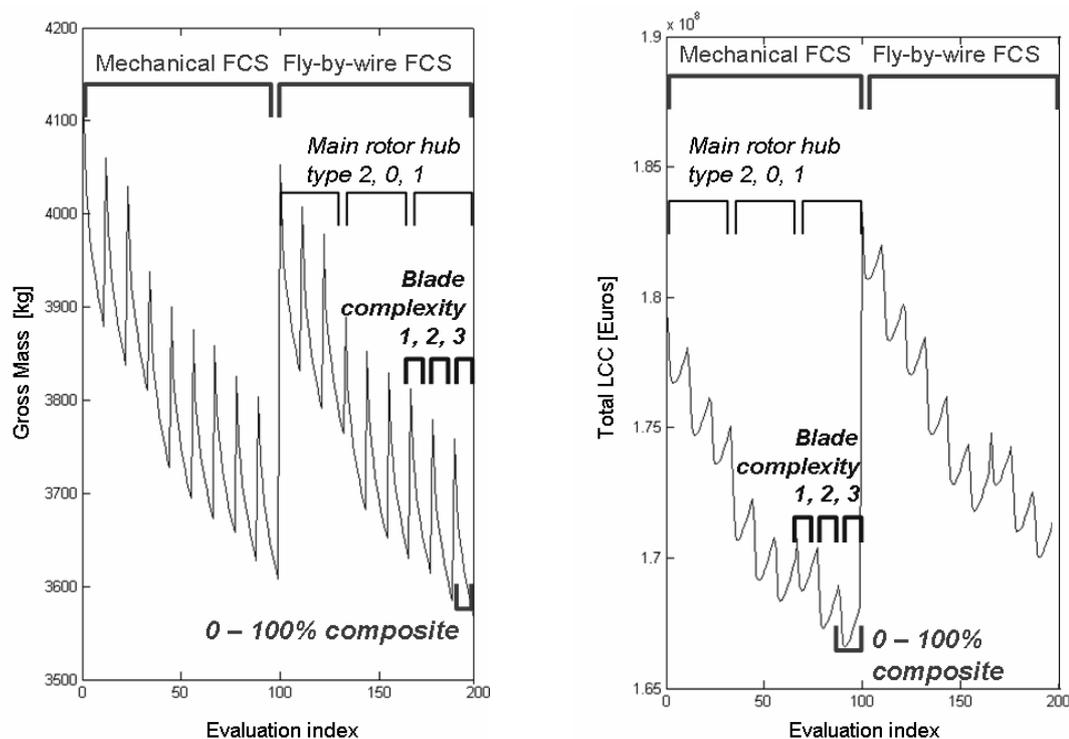
**Fig. 19 Global evaluation of helicopter mass (left) and LCC (right): their dependency on the 4 different design variables**
