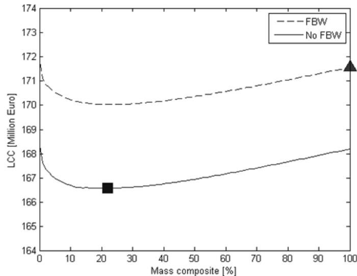
**Fig. 21 Minimum helicopter LCC (square) found for 22 % composite mass in the fuselage and a mechanical flight control system**
