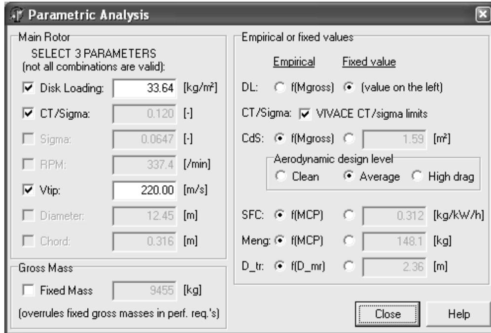
**Fig. 5 Data input form for Parametric Analysis**
