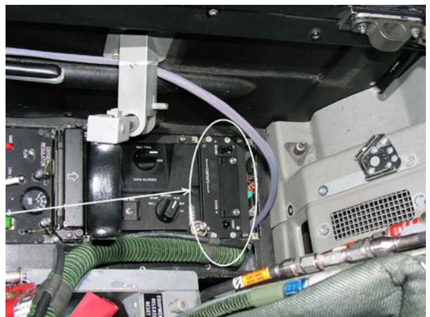
Figure 5: Installation of the recorder in the F-16 cockpit
