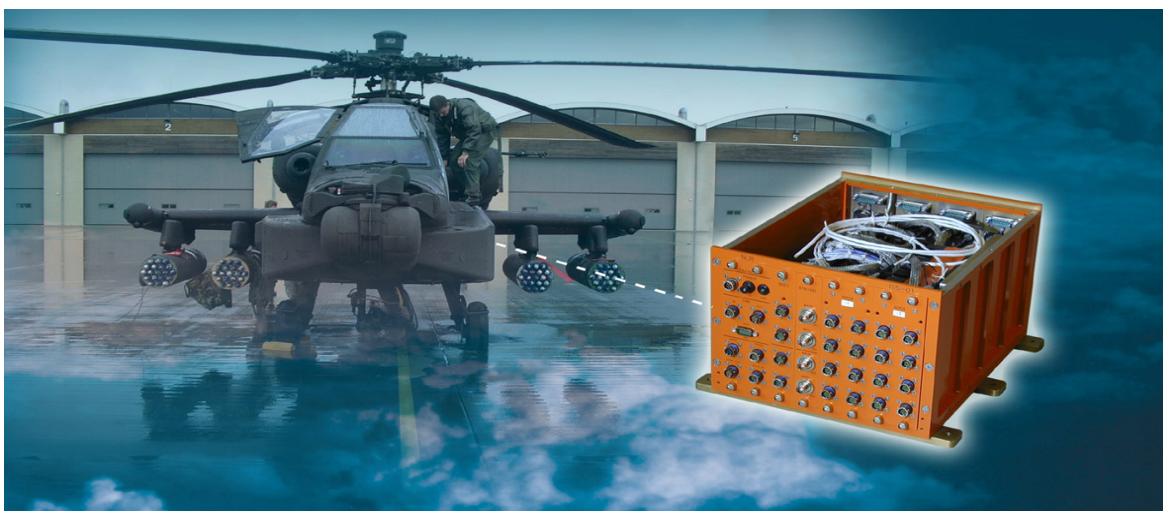
Figure 6: Generic Instrumentation System to be installed for Apache helicopter flight test trials.
