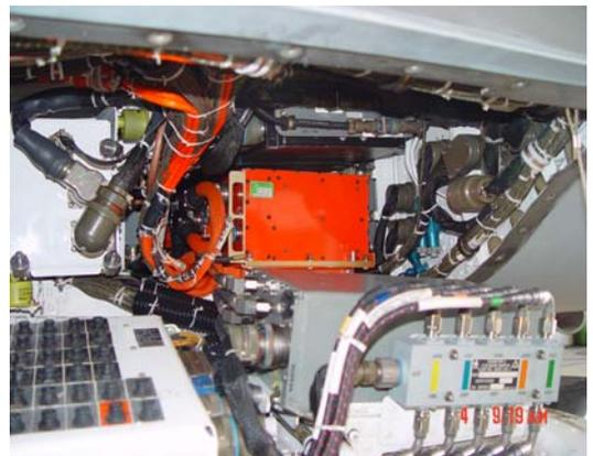
Figure 8 PMU in Aft avionics compartment
