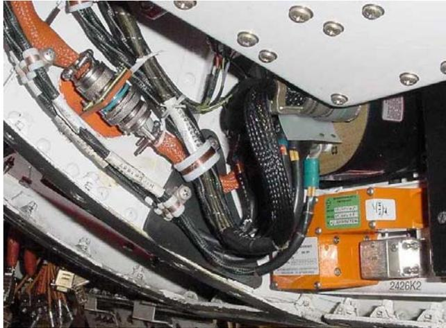
*Figure 4 PCU i/f & transformer behind panel 2304*
