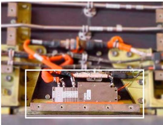
Figure 7 Remote unit at RH side of vertical tail
