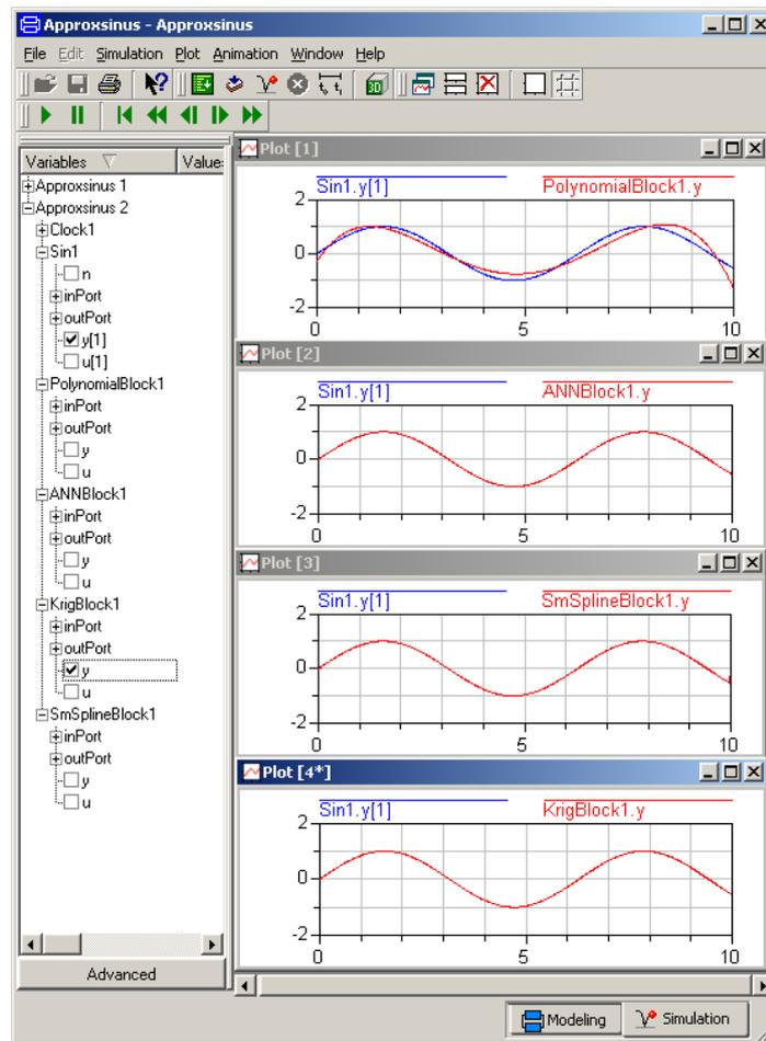
Figure 7 Dymosim simulation results with sinus approximations by (from top to bottom) 4<sup>th</sup> order polynomial, kriging (constant regression Gauss corr.), ANN, smoothing spline.
