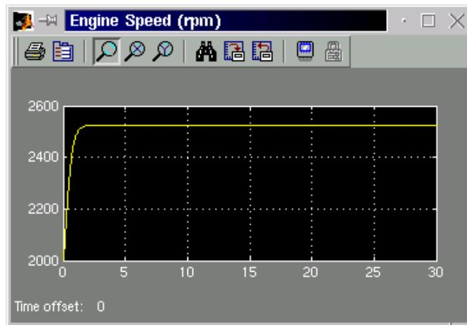
Figure 12 Simulation results for the calculated crank speed (converted to revolutes per minute) with constant torque (20 Nm) and throttle (10 degrees) values
