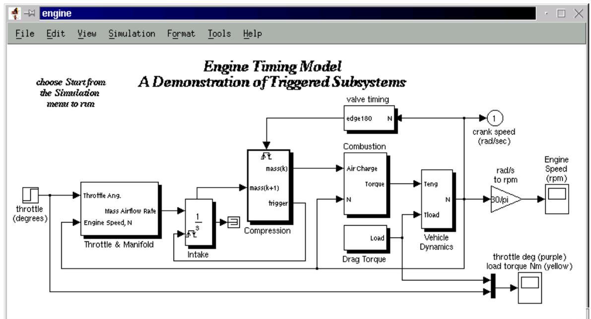
Figure 11 Simulink demo model of an engine [5].
