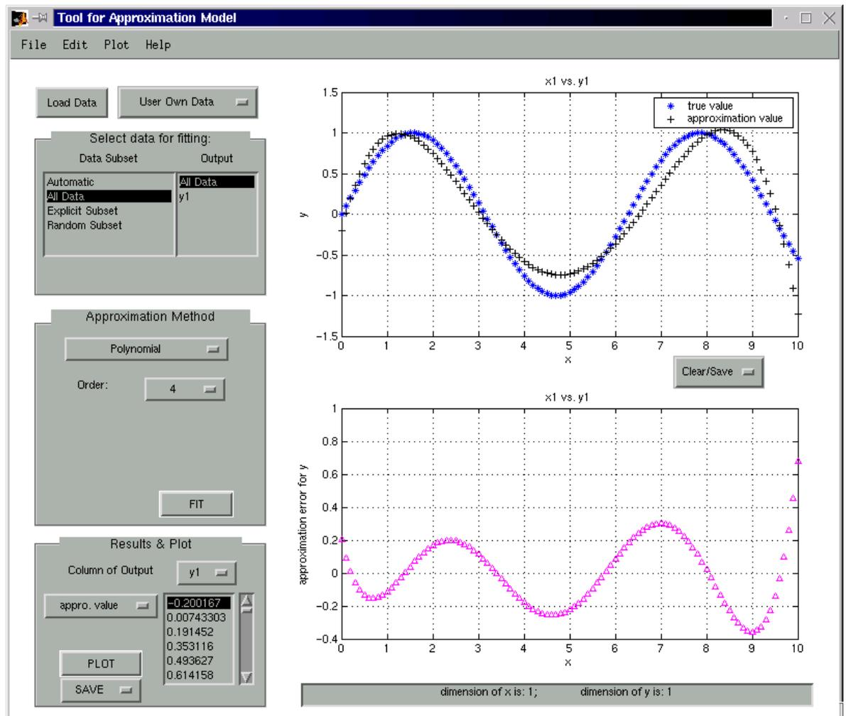
Figure 2 Example of the MultiFit GUI with a 4<sup>th</sup> order polynomial fit to a sinusoidal data set (upper graph in the GUI) and the approximation error (lower graph).
