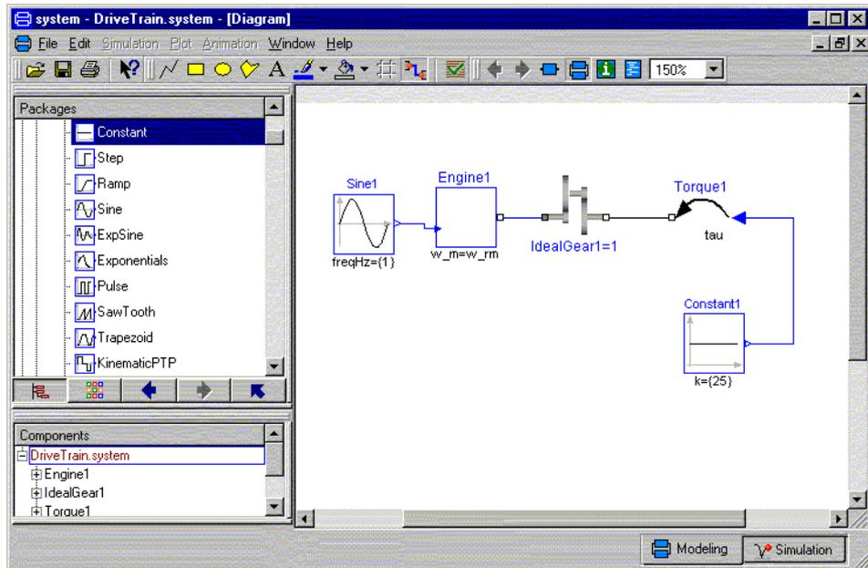
Figure 17 Engine in combination with torque load
