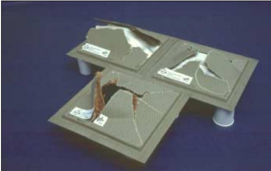
Figure 7 Tensor-skin panels after dynamic impact test (DLR)
