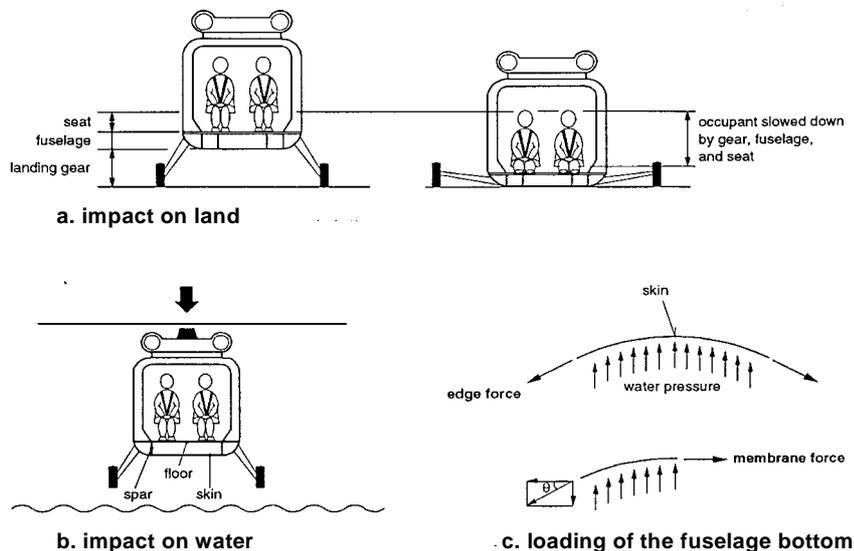
Figure 1 Loading of a sub-floor during water impact
