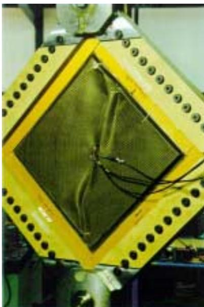
*Figure 5 In-plane shear test on tensor-skin panel*
