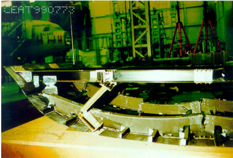
Figure 12 Commuter after impact test (masses are removed) (CEAT)
