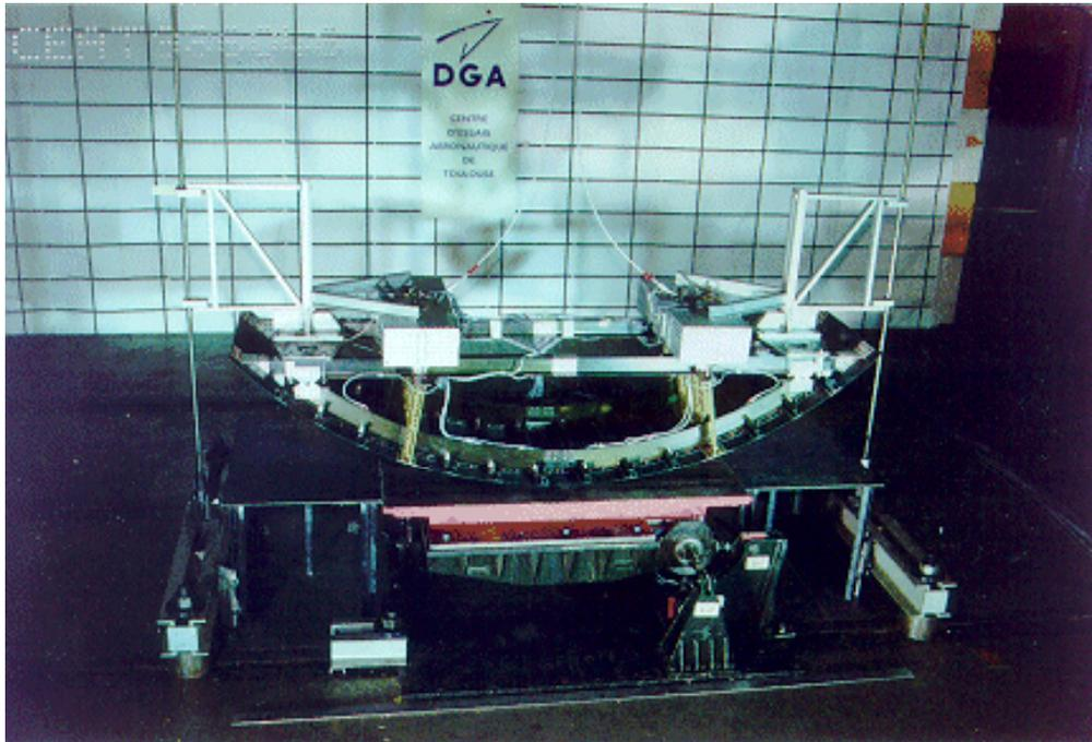
Figure 11 Complete test set-up for dynamic impact test of NLR's commuter (CEAT)
