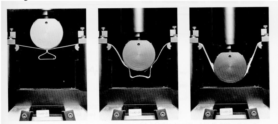
Figure 3 Testing of 1-dimensional tensor-skin specimen made of Dyneema
