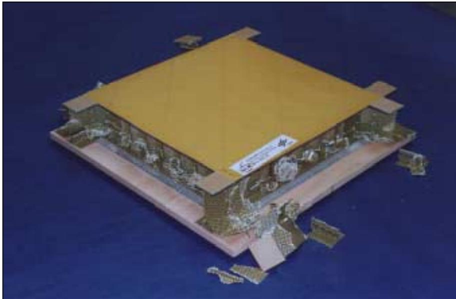
*Figure 9 NLR sub-floor box after dynamic impact (DLR)*
