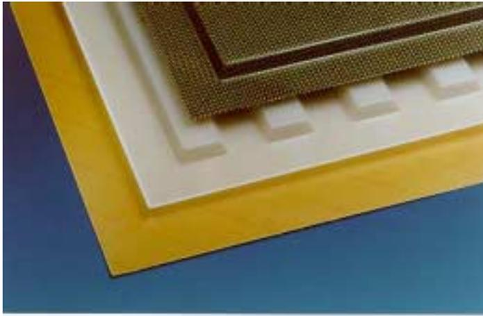
*Figure 4 Lay-up of a tensor-skin panel*
