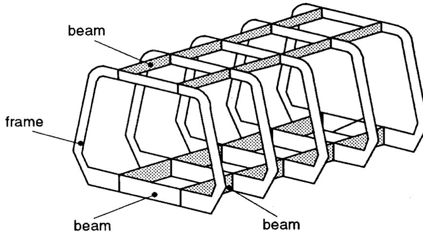
Figure 2 Helicopter structure
