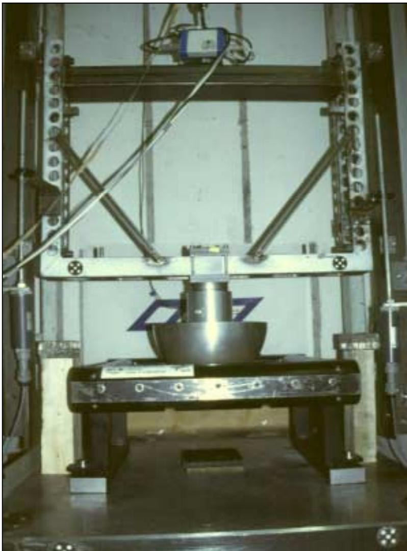
*Figure 6 Test-frame and impact-head in DLR's drop tower*
